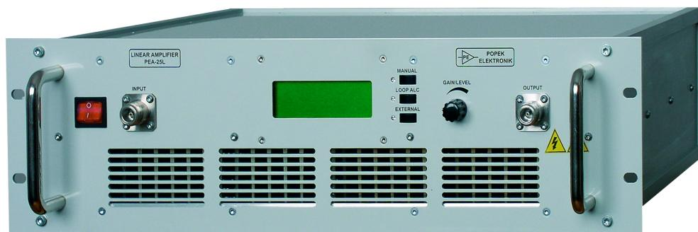
PEA-25L is a linear, broadband telecommunication and, broadband high power amplifier (25 W) making use of automatic measurement systems, broadband telecommunication and laboratories. The broadband and high gain enable the amplifier to gain signals from typical signal generators. After calibration the amplifier with antenna systems are used for generation of electromagnetic measurement fields. The device enables signal transmission with the following modulations: AM, FM, SSB and pulse.
