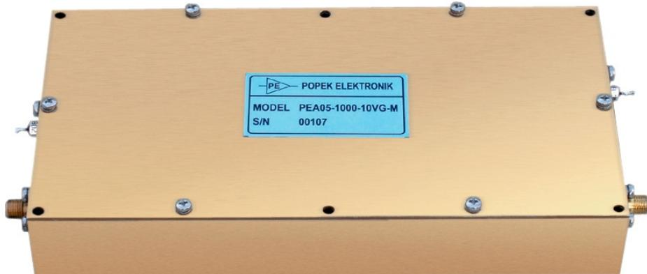
The new, ultra broadband, linear amplifier covers an extremely wide frequency range from 50 kHz to 1000 MHz and provides stable and linear RF power.
